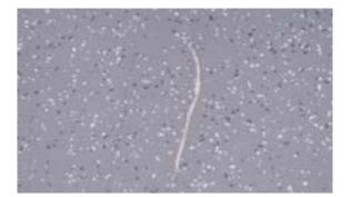
**Step 1)** Clean out the damage by carefully scraping the knife blade along the gouge.
